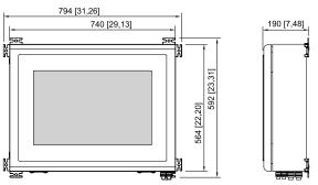
Operator Station FR enclosure, wall mounting
