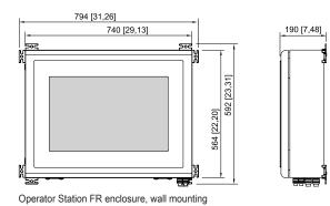
Operator Station CFR enclosure
