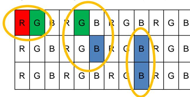
**Distance between Dots**      Definition of distance between two defective dots horizontal, vertical or diagonal, bright or dark (e.g. the following pattern and sub-pixels)
