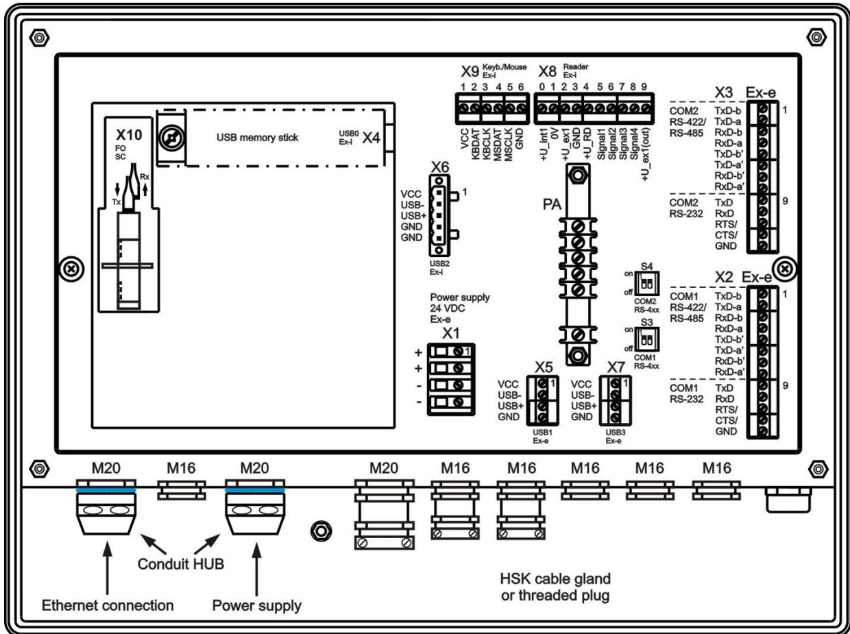
Any cable glands at the operator interface that are not required **MUST BE** replaced by threaded plugs so that the opening in the housing is covered.
