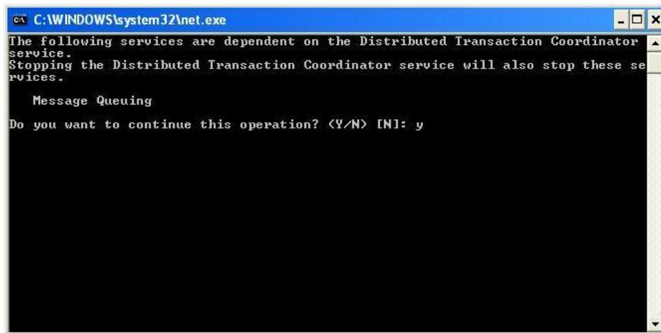
Due to that these MSDTC service is necessary for the SQL Server and the SQL Server is necessary for Siemens WinCC this message **MUST BE** confirmed with **YES** ! Otherwise the MSDTC service will not run.
