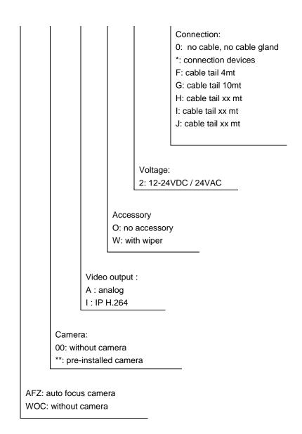
The type code for the Thermal camera frequency is:
