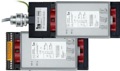
The Digital Output Module Relay Type 9477/12-0\*-12 is an explosion protected electrical apparatus for installation in a Class I, DIV 1 / DIV 2, Groups A, B, C, D or Class I, Zone 1, Group IIC hazardous location according to NEC Article 504/505 or Canadian Electrical Code, CSA C22 that uses relay contacts to control up to eight Non-I.S. circuits.
