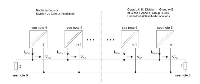
Intrinsically safe RS 485 for Fieldbus connection:
